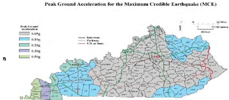
Figure 7-9. Maximum Credible Earthquake (MCE) Median Horizontal Peak Ground Acceleration for the Commonwealth of Kentucky, Site Class A (Hard Rock)
